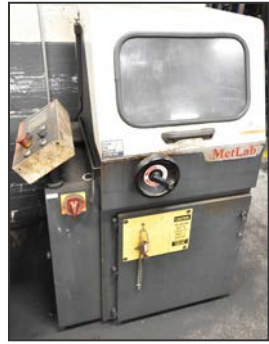
METLAB MET500H enclosed cut off saw
