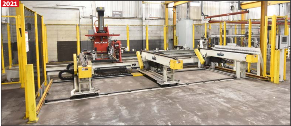
LINCOLN ELECTRIC AUTOMATION/TRUAXIS AD2490 TRUAXIS straightening system
