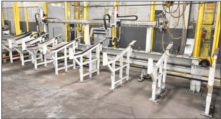
View of bar stacking stands
