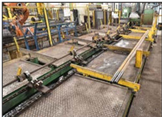
View of bar loading conveyor
