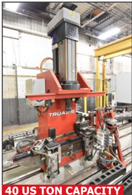
Close up of view of TRUAXIS pneumatic press
