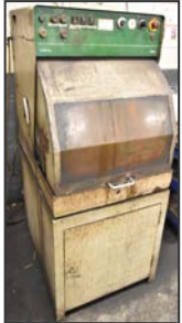
EXOTOM STRUERS enclosed cut off saw
