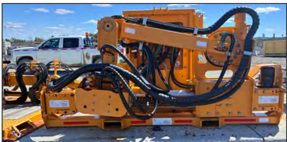
MCCLEAN trailer mount drill rig
