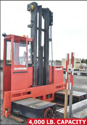
RAYMOND 71-SL40TT SIDELOADER 36V electric forklift
