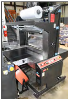
DAMARK B34MP-16 shrink auto wrap bundling system
