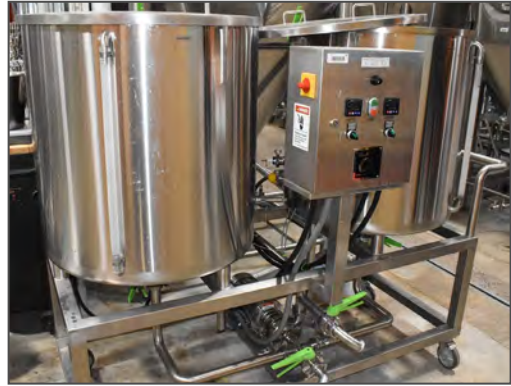
ALPHA C.I.P. stainless steel portable clean-in-place system
