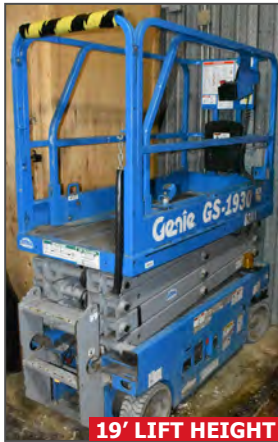
GENIE GS-1930 500 LB. capacity 24V electric scissor lift
