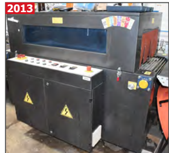
2013 SHRINK PACKAGING EQUIPMENT SM-6530LX heat shrink tunnel
