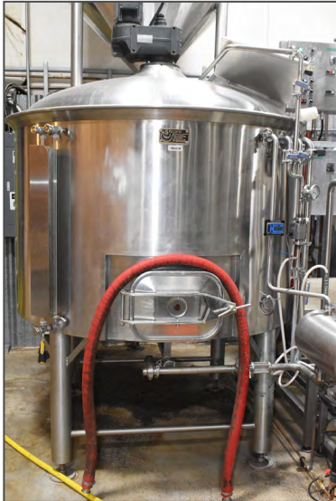
SPECIFIC MECHANICAL SYSTEMS 548 gal. capacity SS jacketed mixing brew kettle
