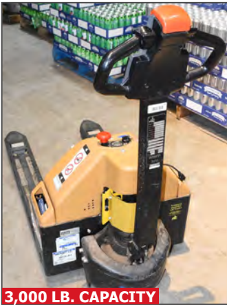
BIG JOE E-30 24V electric walk-behind pallet truck
