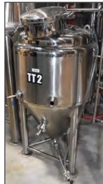
Stainless steel jacketed pilot batch fermenting tank
