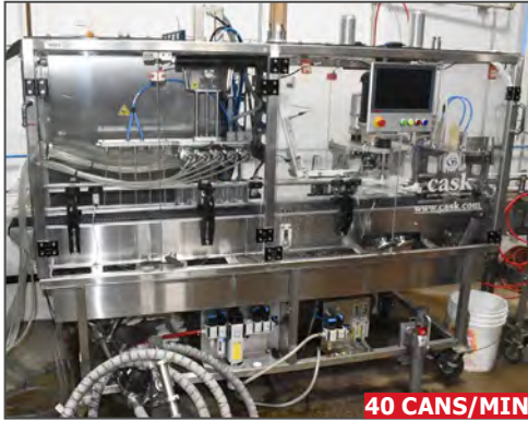
CASK GLOBAL CANNING SOLUTIONS ACS MOBILE compact portable automatic 5-head can filler
