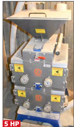
5 HP SASQUATCH 4-roll malt roller mill
