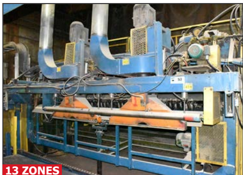
COE L353 4 level natural gas veneer dryer
