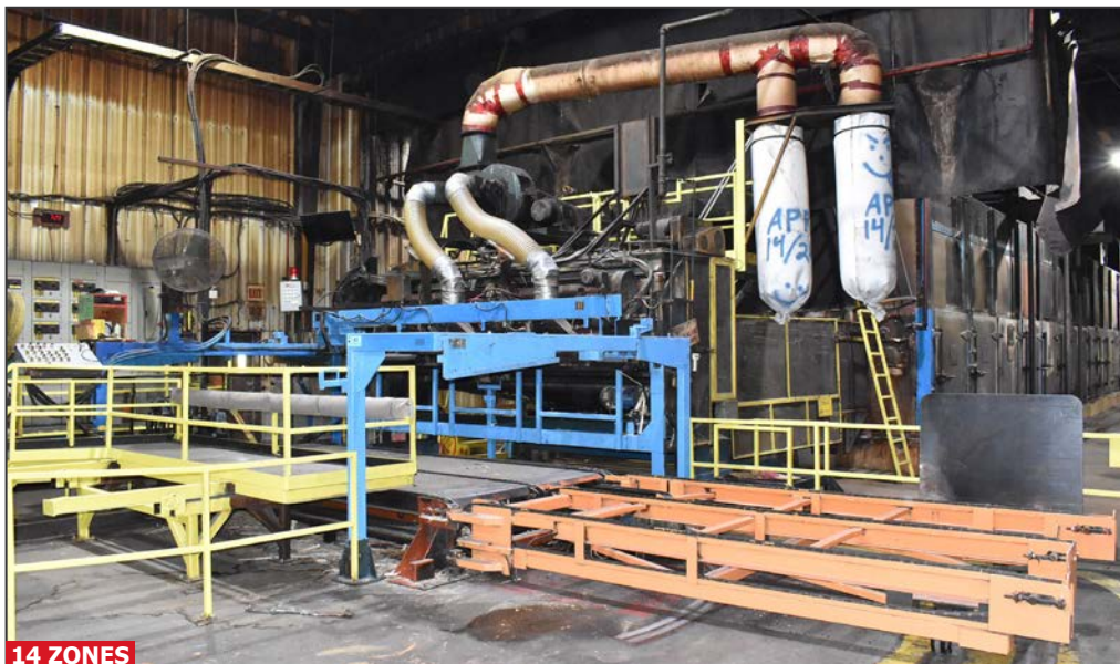
COE L353, 4 level natural gas veneer dryer
