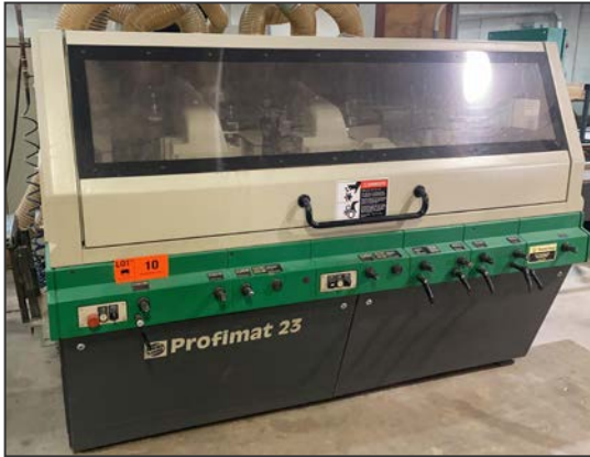
WEINIG PROFIMAT P23 6-head feed through moulder
