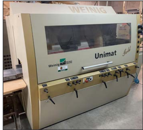
WEINIG UNIMAT U GOLD 6-head feed through moulder
