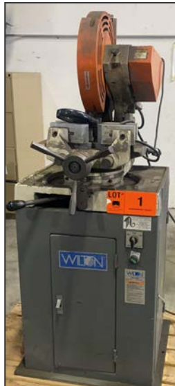
WILTON CK350-2 conventional cold cut saw
