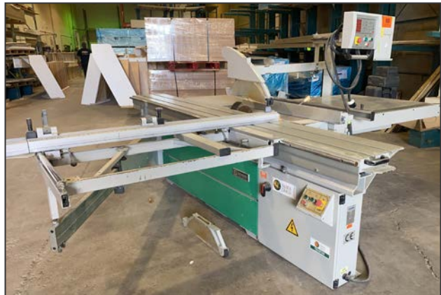
BOSS P-3200TA sliding table saw
