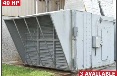
40 HP AEROVENT SCDW-1250-593-40 industrial air make up unit
