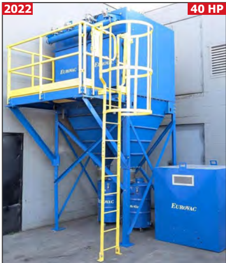
EUROVAC CPA-401-83AP0262 cartridge-type industrial central dust collector
