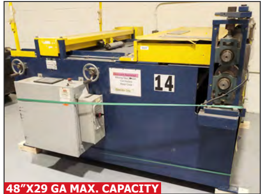
METAL ROLL FORMING SYSTEMS automatic coil fed cut-to-length system
