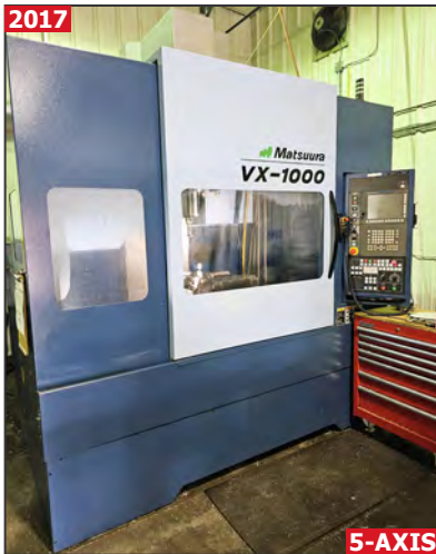
MATSUURA VX-1000 MAXIA 5-axis CNC high speed vertical machining center
