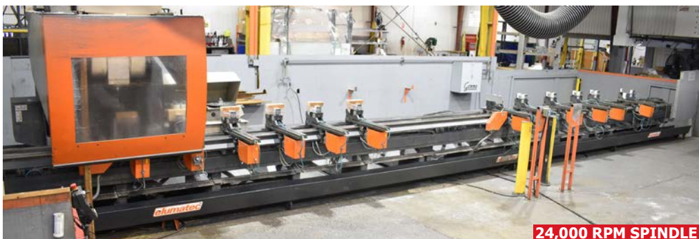
ELUMATEC SBZ150 5-axis CNC profile machining center
