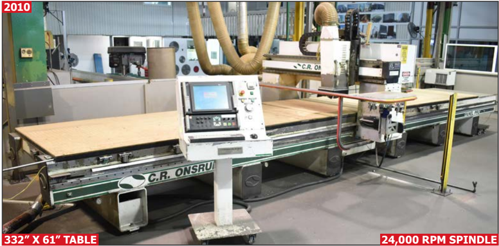
C.R. ONSRUD 288G25 CNC bride type router table
