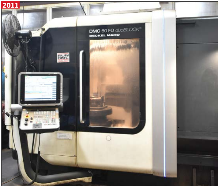
DECKEL MAHO DMC60 FD DUOBLOCK 5-axis high speed twin pallet CNC vertical machining center
