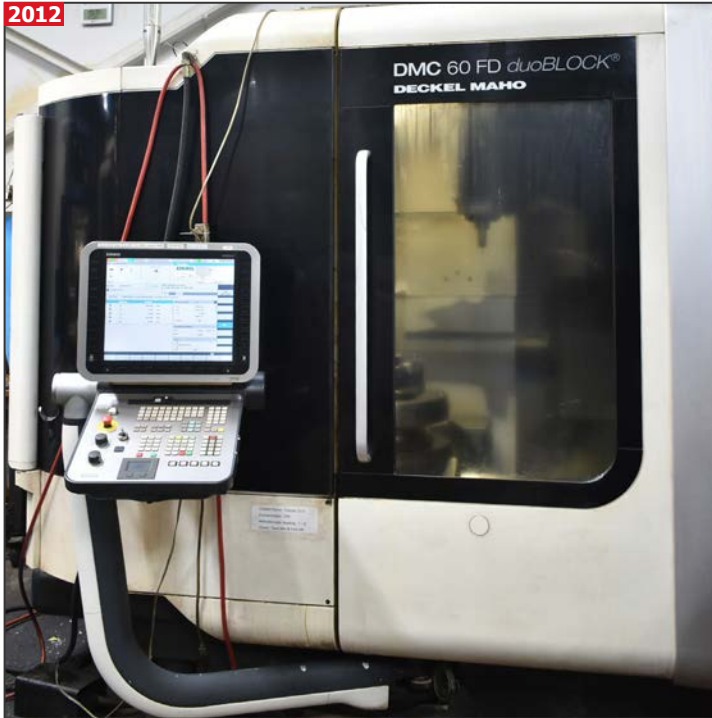
DECKEL MAHO DMC60 FD DUOBLOCK 5-axis high speed twin pallet CNC vertical machining center
