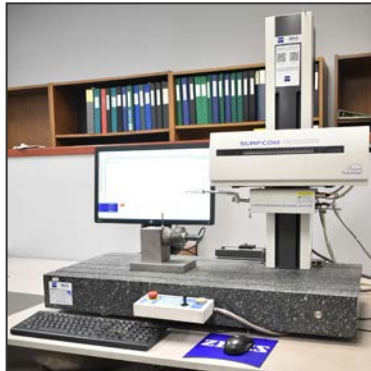
LINEAR TECHNOLOGY SURFCOM 1900SD3 contour measuring detector instrument
