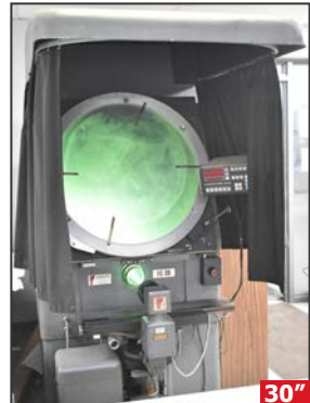
JONES & LAMSON FC-30 floor-type optical comparator
