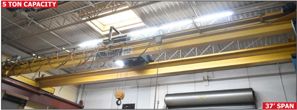
MUNCK LOADRUNNER double girder top-running overhead bridge crane
