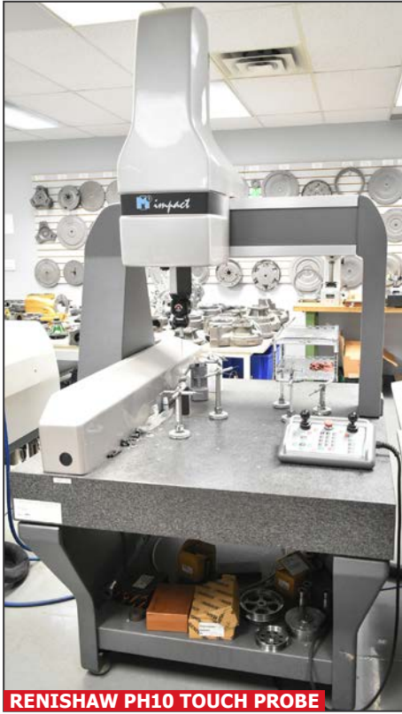
RENISHAW PH10 TOUCH PROBE IMS IMPACT coordinate measuring machine
