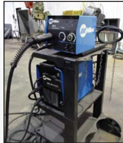
MILLER XMT 350 mig welder with wire feed
