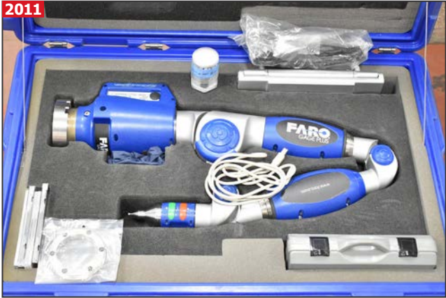
2011 FARO F04 GAUGE PLUS 6-axis portable co-ordinate measuring arm
