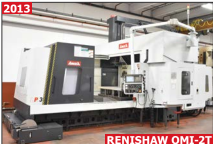
AWEA LP-3016YF CNC multi-face bridge type CNC vertical machining center
