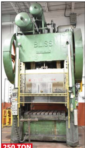
BLISS S2-250-60-42 double crank SS mechanical stamping press
