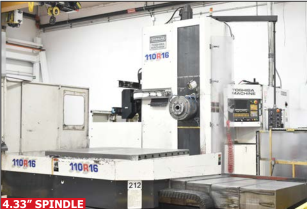
TOSHIBA SHIBAURA LTD-110.R16 CNC table-type horizontal boring mill
