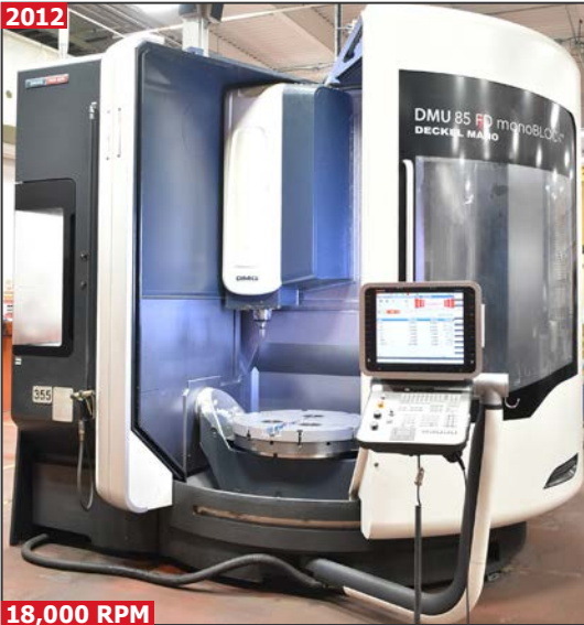
DMG MORI DMU 85 FD MONOBLOCK 5-axis high speed CNC vertical machining center
