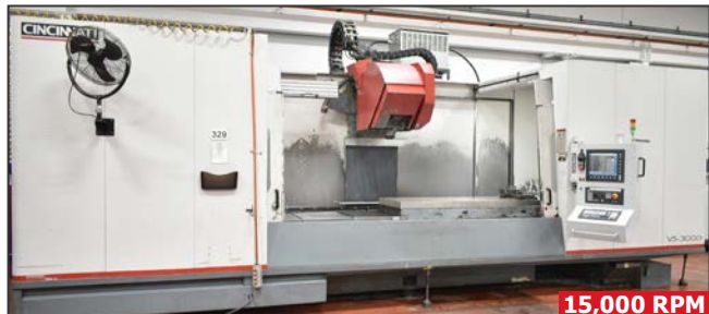
CINCINNATI V5-3000 5-axis high speed CNC vertical machining center
