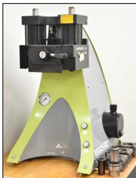
REGO-FIX POWRGRIP PGU9000 HSK 63 clamping tool pre-setter
