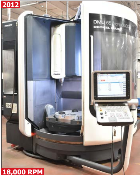
DMG MORI DMU 65 MONOBLOCK 5-axis high speed CNC vertical machining center
