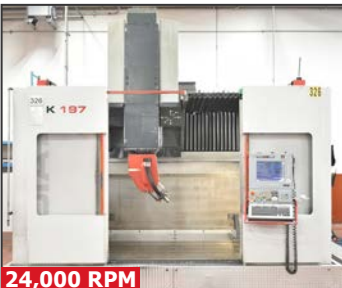
FIDIA K197/5 5-axis high speed CNC vertical machining center
