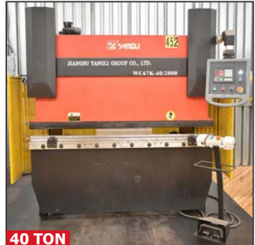
JIANGSU YANGLI WC67K-40/2000 CNC hydraulic press brake
