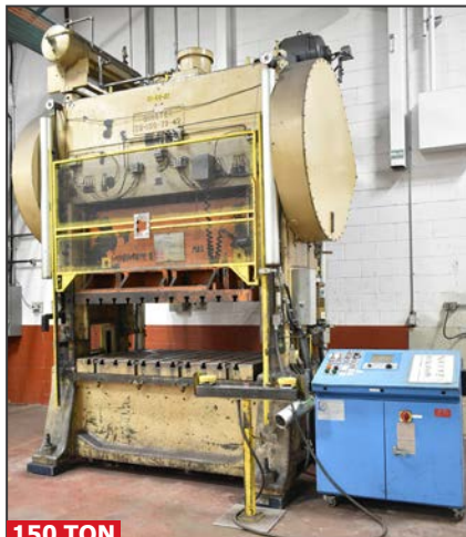
MINSTER S2-150-72-42 double crank straight side mechanical stamping press
