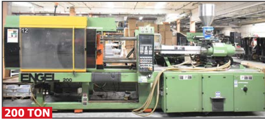
ENGEL ES150/200BH horizontal plastic injection molding machine
