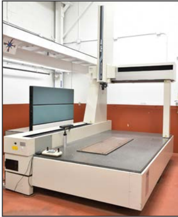
MITUTOYO BRT-A1220 BRIGHT APEX co-ordinate measuring machine
