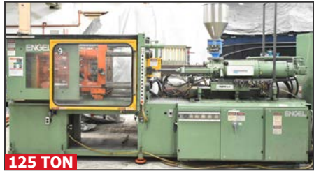
ENGEL ES600/125 horizontal plastic injection molding machine
