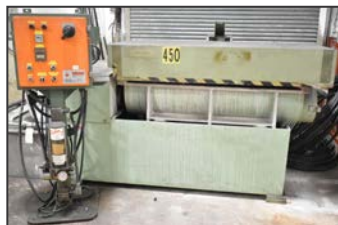
VIBRAFINISH VF-6.50 tub-style vibratory finisher
