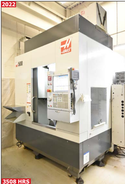
HAAS UMC-500 5-axis high speed CNC vertical machining center
