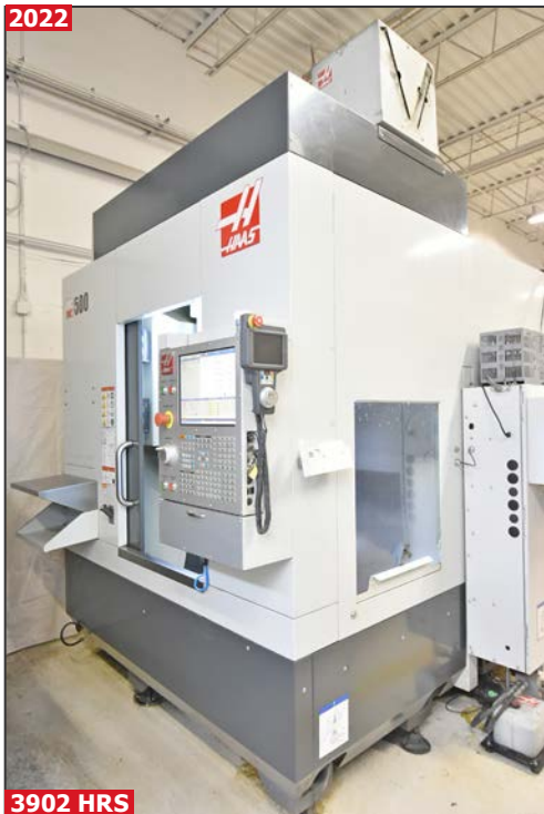
HAAS UMC-500 5-axis high speed CNC vertical machining center
