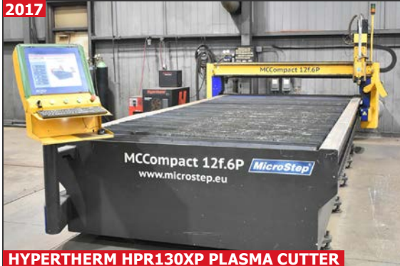
MICROSTEP RS MASTER CUT COMPACT 12F.6P CNC plasma cutting machine
