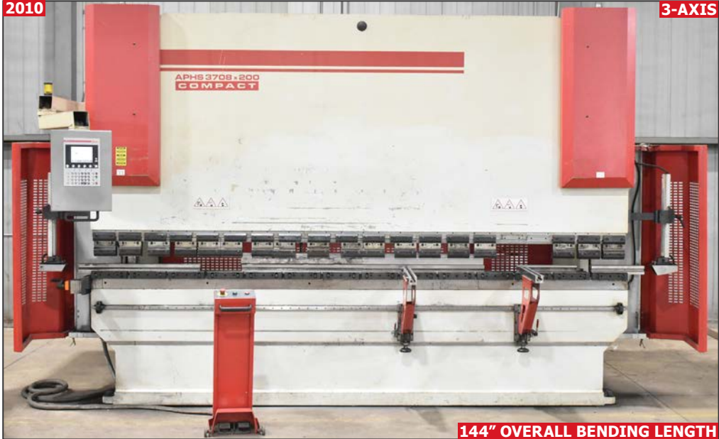
BAYKAL APHS 3708X200 COMPACT 200 ton capacity CNC hydraulic press brake
