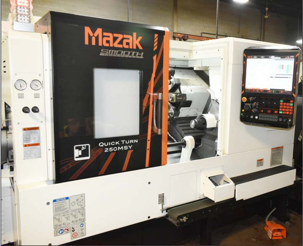
MAZAK QUICK TURN 250MSY CNC opposed spindle multitasking center
