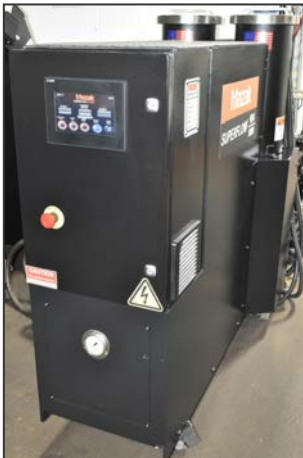
MAZAK SUPERFLOW V8A/1000 high pressure coolant system (250MSY)
