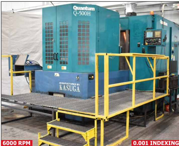
KASUGA Q-500H twin pallet horizontal CNC machining center
