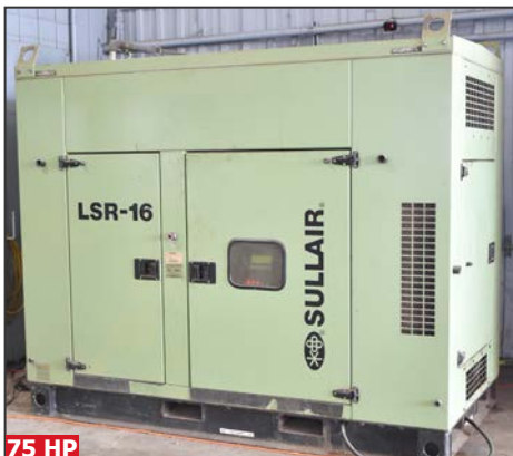
SULLAIR LSR16-75 AC 75 HP rotary screw air compressor
