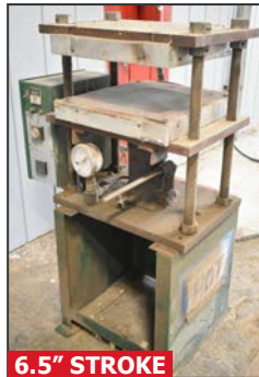
CARVER 25 ton capacity manual heated press
