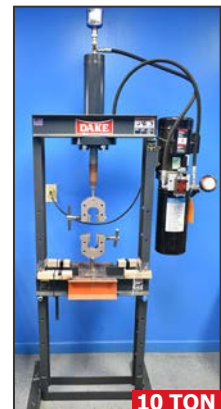
DAKE MODEL 909205 hydraulic tension tester
