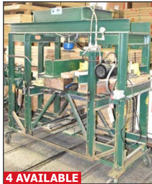
GBT CUSTOM hydraulic destructive panel tester
