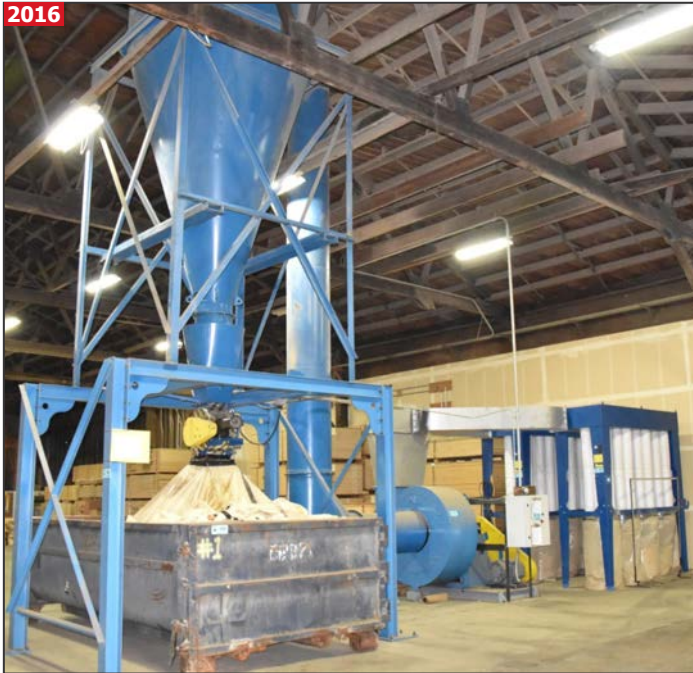
DONALDSON cyclonic type plant dust collection system
