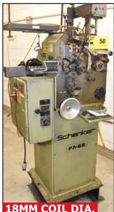
18MM COIL DIA. SCHENKER FA-6S spring coiling machine
