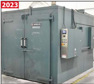
2023 GRIEVE WRC686-500 60 kW electric convection oven
