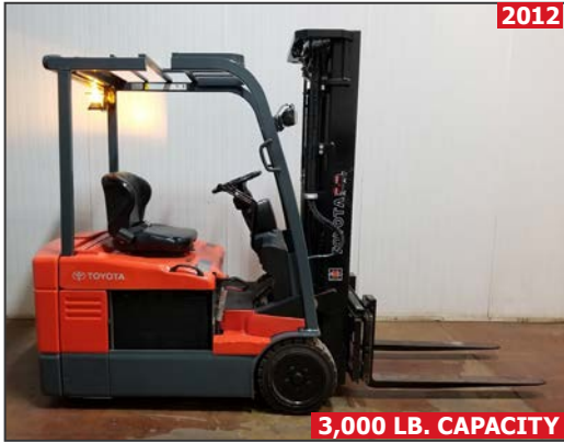
TOYOTA 7FBEU18 electric counterbalance forklift
