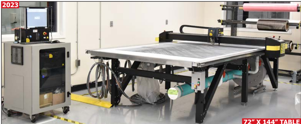
LECTRA GERBER TECHNOLOGY DCS 2600 high speed low ply cutting CNC system
