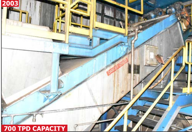
METSO 140-04 stainless steel inclined twin screw press
