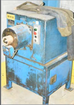
LAR MACHINERIE 2461-S core cap hydraulic crimper
