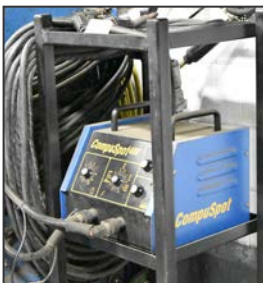
COMPU SPOT CPS-400 16KVA portable spot welder
