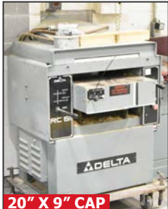
20" X 9" CAP DELTA RC51 heavy duty floor type planer
