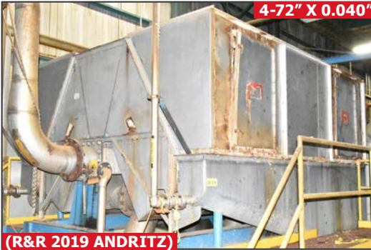
CE BAUER MODULAR HYDRASIEVE MODEL 552 SS vertical de-watering screen
