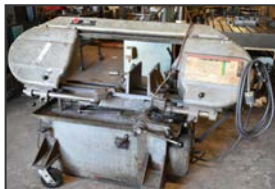
ER MAIER KM1012 horizontal band saw
