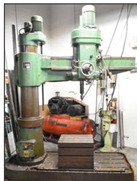
MAS Z35 6' radial arm drill
