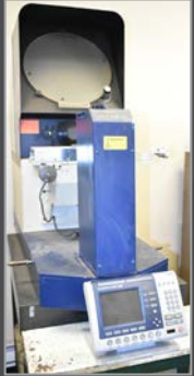
MITUTOYO 612TS optical comparator
