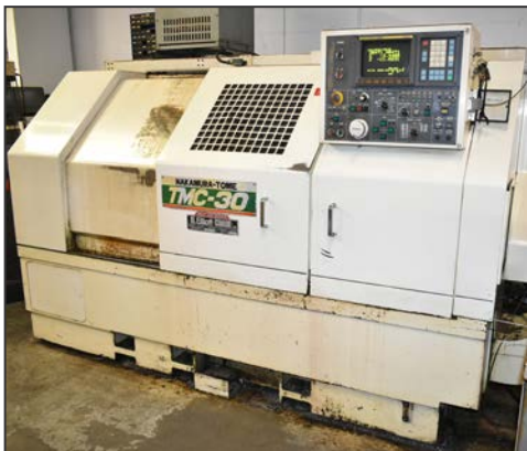
NAKAMURA TOME TMC-30 CNC turning center
