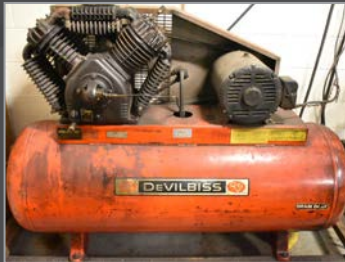
DEVILBISS 15HP piston type air compressor
