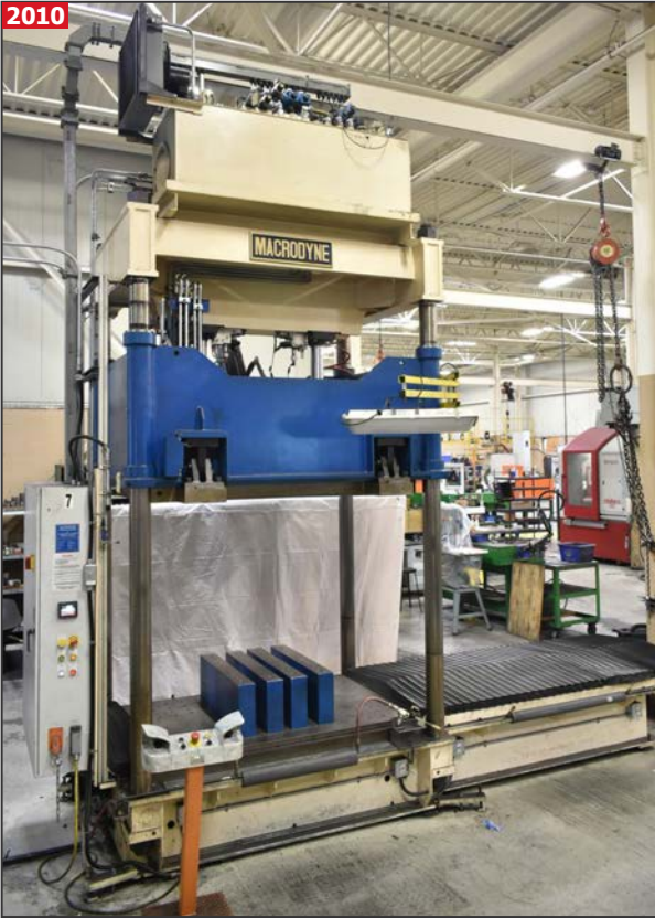
MACRODYNE MPS-50 50 TON 4 post hydraulic spotting press
