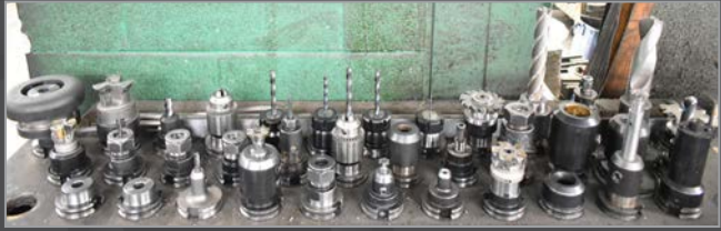
Partial view of 40 taper tool holders available
