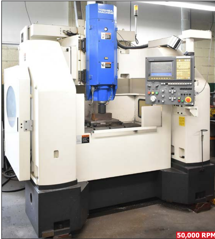
TOSHIBA ASV400 high speed CNC vertical machining center
