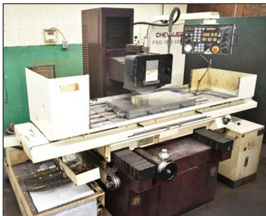
CHEVALIER FSG-1632 ADII hydraulic surface grinder
