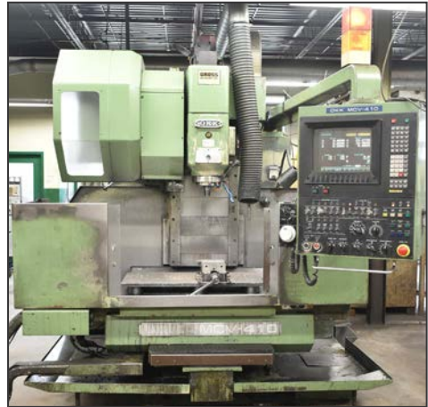
OKK MCV-410 CNC vertical machining center
