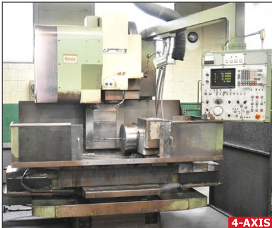
4-AXIS MORI-SEIKI MV35/40 CNC vertical machining center
