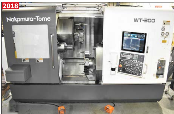
NAKAMURA-TOME WT-300 multi-axis opposed spindle and twin turret CNC multi-tasking center
