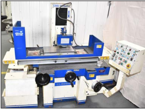
CLAUSING CSG-1020ASD hydraulic surface grinder
