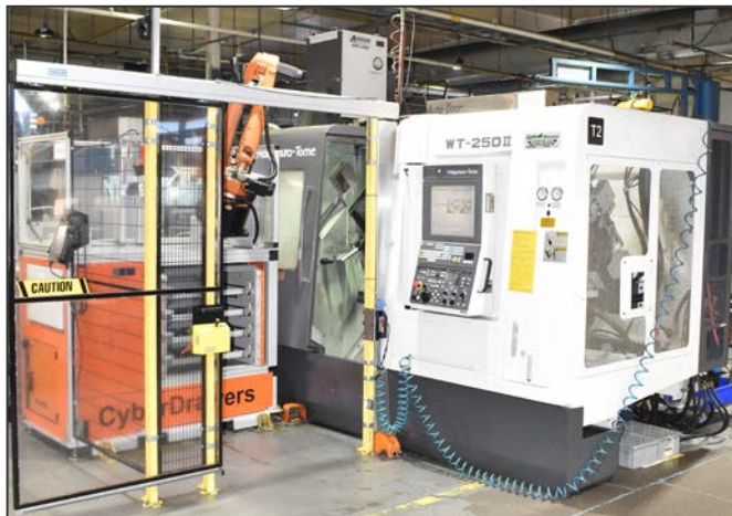
NAKAMURA-TOME WT-250 II multi-axis opposed spindle and twin turret CNC multi-tasking center
