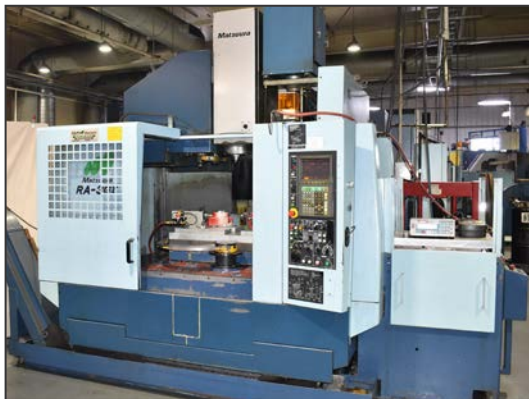
MATSUI RA-3G2 4-axis twin-pallet high-speed CNC vertical machining center
