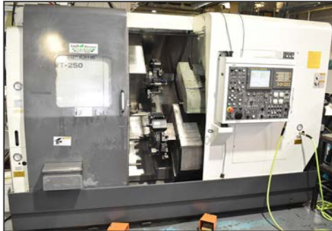
NAKAMURA-TOME WT-250 multi-axis opposed spindle and twin turret CNC multi-tasking center
