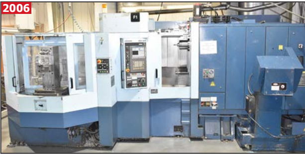
MATSUURA H.PLUS-405 4-axis multi-pallet high-speed CNC horizontal machining center
