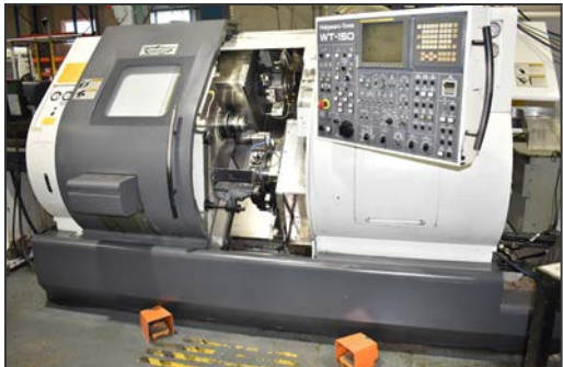
NAKAMURA-TOME WT-150 multi-axis opposed spindle and twin turret CNC multi-tasking center
