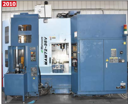
MATSUURA MAM72-35V high-speed CNC vertical machining center
