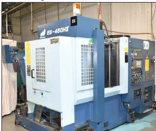
MATSUI ES 450 H2 twin-pallet high-speed CNC horizontal machining center
