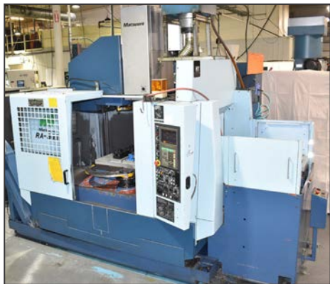
MATSUI RA-3G2 twin-pallet high-speed CNC vertical machining center
