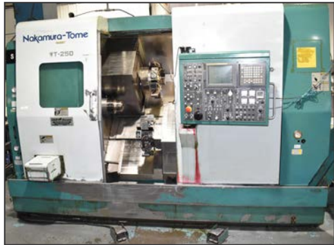
NAKAMURA-TOME WT-250 multi-axis opposed spindle and twin turret CNC multi-tasking center
