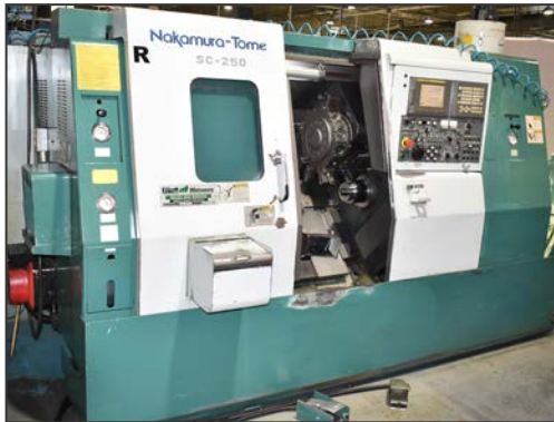
NAKAMURA-TOME SC-250 opposed spindle CNC turning center
