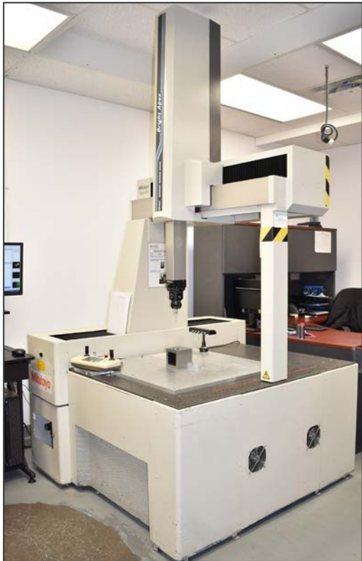
MITUTOYO BRT-A707 BRIGHT APEX coordinate measuring machine
