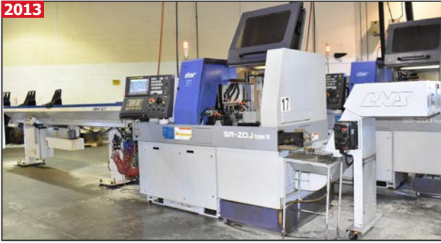
STAR SR-20J TYPN N 7-axis CNC SWISS type high speed automatic lathe
