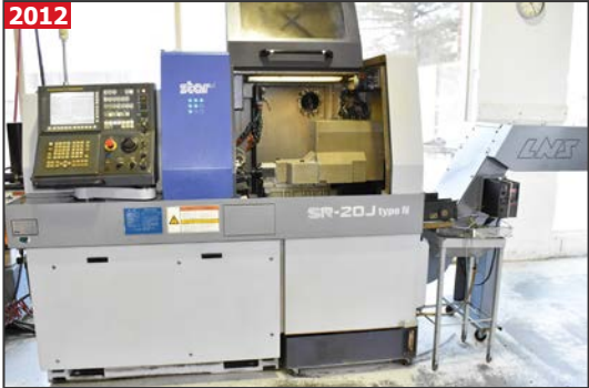
STAR SR-20J TYPN N 7-axis CNC SWISS type high speed automatic lathe
