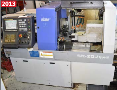
STAR SR-20J TYPN N 7-axis CNC SWISS type high speed automatic lathe
