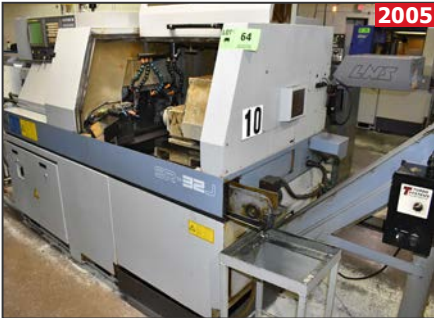
STAR SR-32J 7-axis CNC SWISS type high speed automatic lathe
