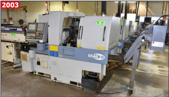
STAR ECAS 20 CNC 7-axis SWISS type automatic high speed lathe
