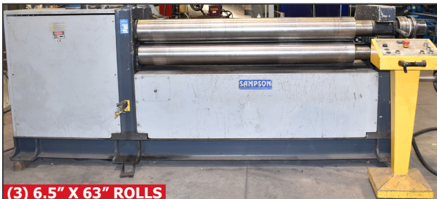
SAMPSON (2002) MRS560 1/4" thick plate bending rolls
