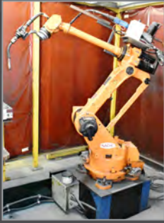
NACHI SC06F-02 robotic welding cell
