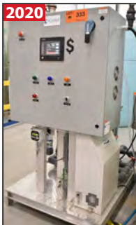
ACLARUS skid-mounted ozone system
