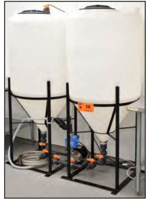
Dual tank mixing system
