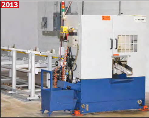
FH MACHINERY THC-B70NC fully automatic high speed CNC circular cold cut saw
