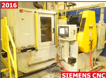
C&B SDG6-42 CNC horizontal double disk grinder
