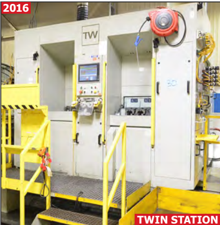
TRI-WAY OP10 4-axis CNC horizontal machining center
