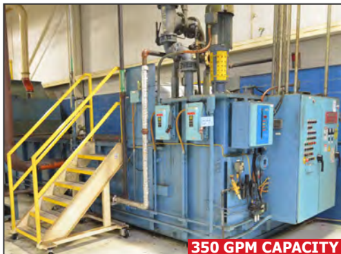
HENRY centralized coolant filtration system
