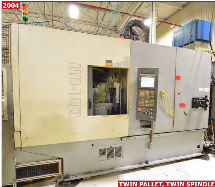
CHIRON DZ 15K W MAGNUM high speed 5-axis CNC machining center
