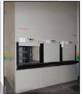
KARDEX INDUSTRIEVER 8000 automated storage system
