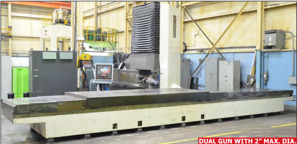
DUAL GUN WITH 2" MAX. DIA. TPI TARUS TPTCGD512 4 axis CNC dual spindle table-type gun drill
