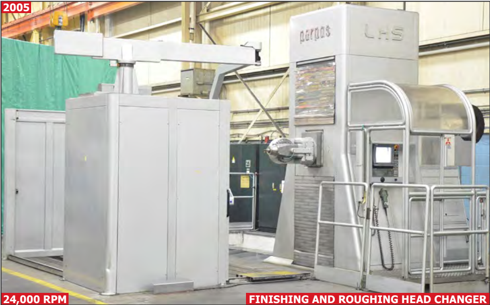
24,000 RPM FINISHING AND ROUGHING HEAD CHANGER PARPAS LHS 5 axis floor-type CNC universal boring/milling machine
