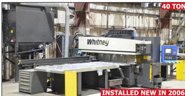
WHITNEY 3400 XP CNC combination punch/plasma with hypertherm HYSPEED HT2000LHF plasma cutter
