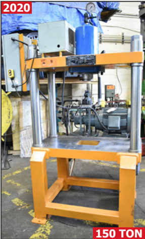
ALKANO MODEL HP 4P 33/19 4-post hydraulic stamping press
