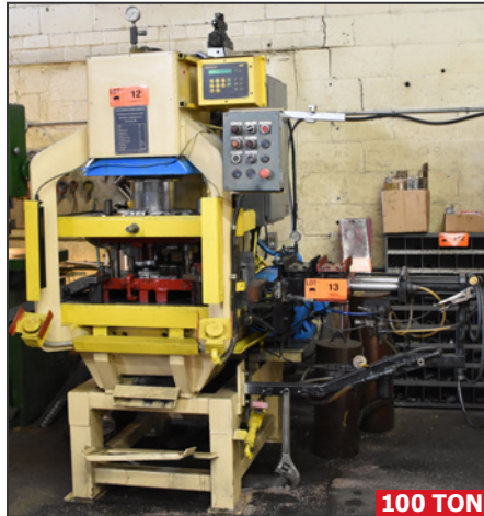
ALKANO MODEL CF100 c-frame hydraulic stamping press
