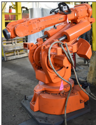
ABB IRB 6400 FOUNDRY PLUS 6 axis industrial robot
