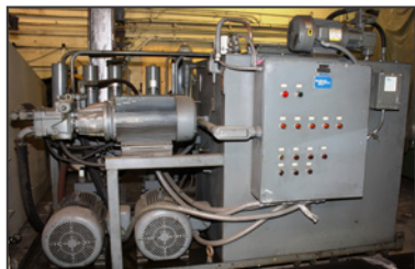
BEHCO 120HP heavy-duty hydraulic power pack
