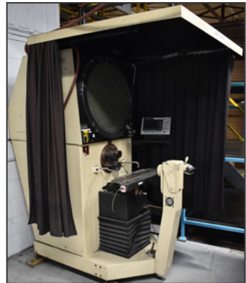
ST INDUSTRIES MODEL 20-2450 24" optical comparator
