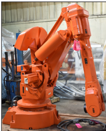
ABB IRB 6400 FOUNDRY PLUS 6 axis industrial robot
