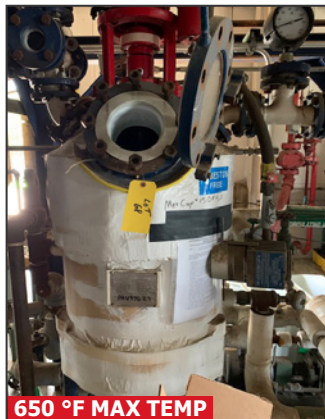
CERAMIC COATING CO. glass lined reactor with agitator
