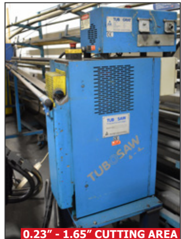
TRACTO-TECHNIK TUBOSAW w/ TRACTO-TECHNIK TUBOGRAT deburring machine
