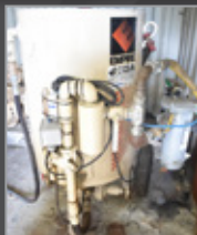
EMPIRE SUPER-P650-7P portable pot-type sand blaster
