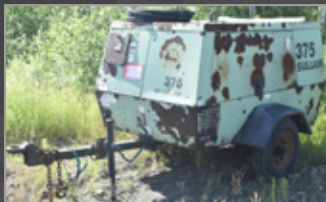
SULLAIR 375 DPQ JD 113 HP tow-behind air compressor
