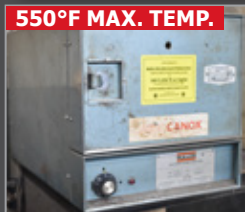
GULLCO MODEL 125 benchtop electrode stabilizing oven
