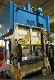
**FEATURING:** BLOW (1998) SC2-200-72-42, 200 ton straight side double crank stamping press with 42" x 72" bed, 8" stroke, 24" shut height, 8" ram adjustment, 40-80 SPM, 30HP drive, windows, light curtains, S/N SDG-200-463-98; MECON servo press feedline consisting of: MECON 400F-24 THD servo press feeder; MECON 200GC-PR, servo straightener/feeder; MECON 200BTJ36, 20,000lb uncoiler with coil car
