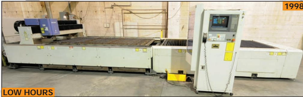
Overall view of MITSUBISHI ML3015LXP 2000 WATT flying optic CNC laser
