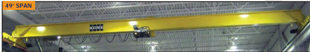
KONE 5 ton single girder underslung bridge crane
