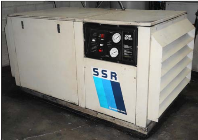
INGERSOLL-RAND SSR EP-50 50 HP rotary screw air compressor
