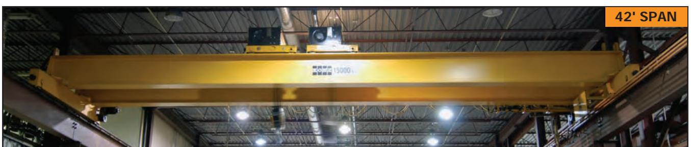
KONE 10 ton double girder, top running bridge crane with 15 ton auxiliary hoist
