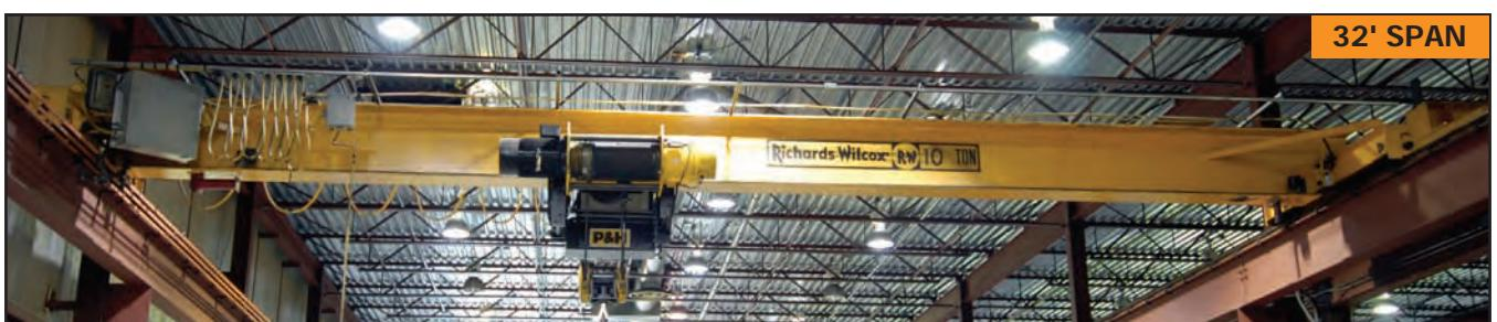
RICHARDS WILCOX 10 ton single girder, underslung, bridge crane
