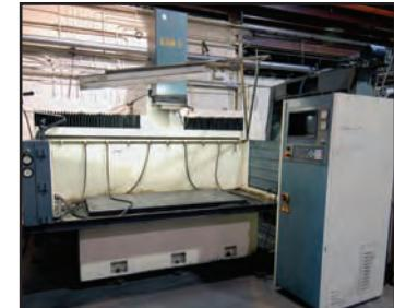
**JSEDM** NCF9091/120A ram type EDM**2004**
