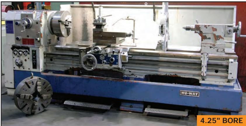
NU WAY 27"/37" X 84" gap bed engine lathe
