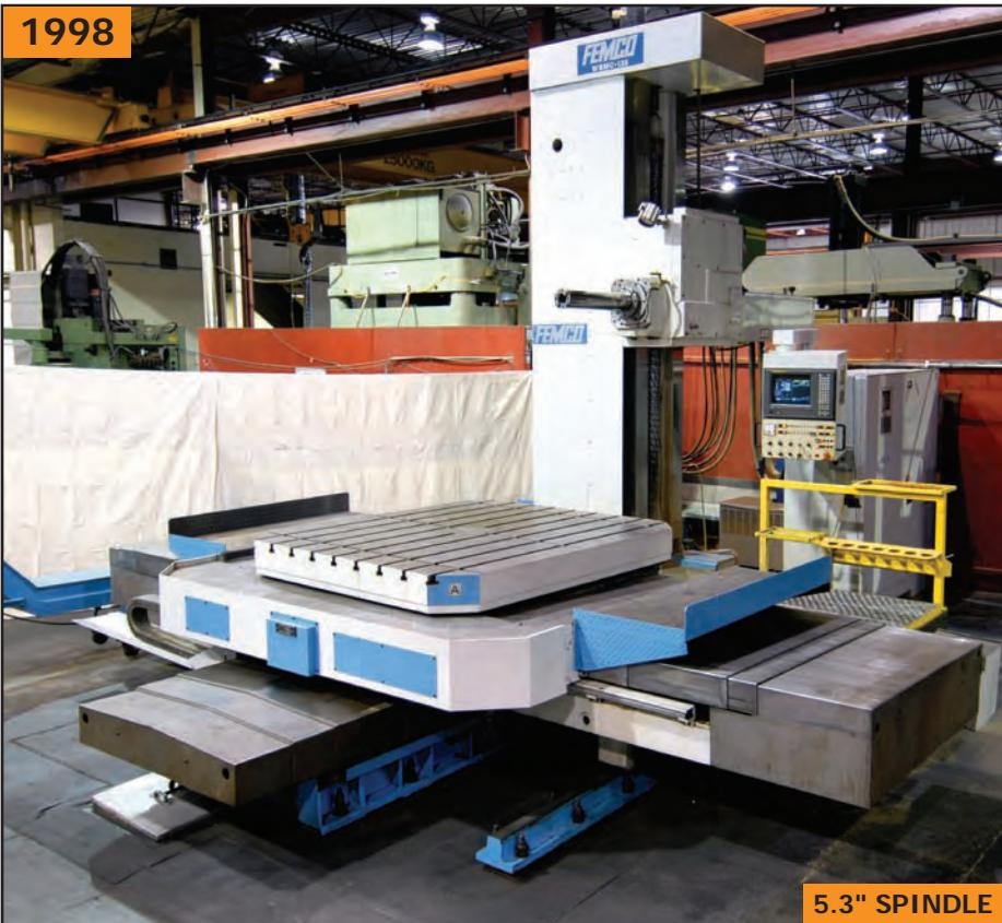
FEMCO BMC 135 CNC table type horizontal boring mill
