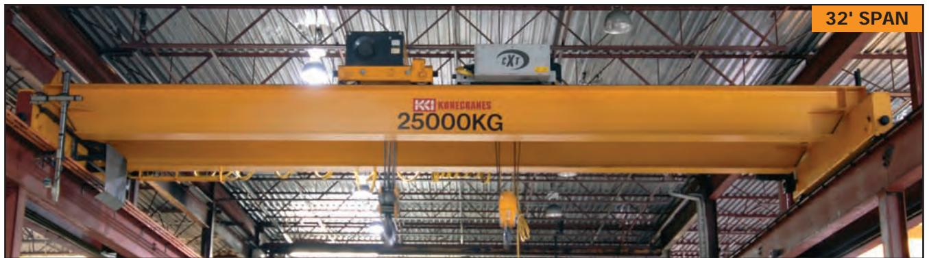
KONE 25 ton double girder, top running bridge crane with 20 ton auxiliary hoist
