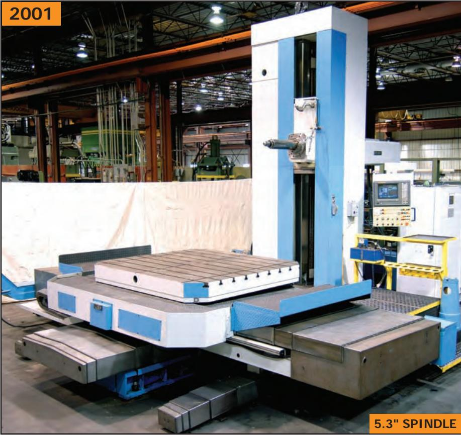
FEMCO BMC 135 CNC table type horizontal boring mill
