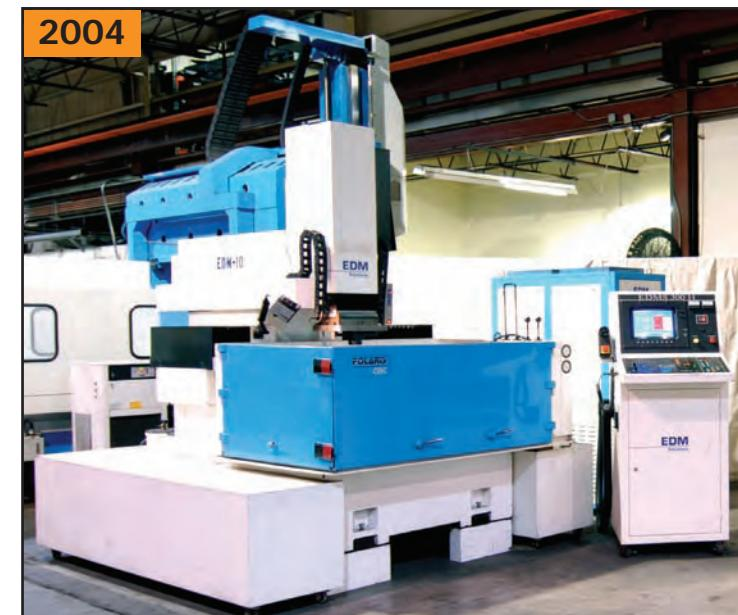
**EDM SOLUTIONS** POLARIS CNC ram type EDM**2004**
