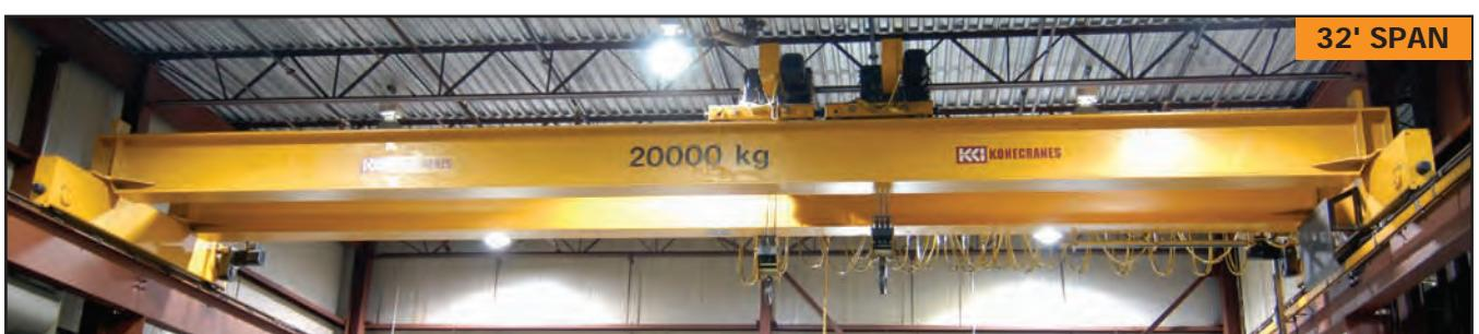
KONE 20 ton double girder, top running bridge crane with 15 ton auxiliary hoist
