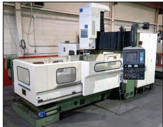
**KAO MING** KMC-2000S CNC double column vertical machining center
