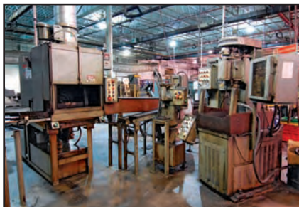
View of BE STR 233 balancer, press and ROSS DETROIT 3-36H hyd broach oven cell
