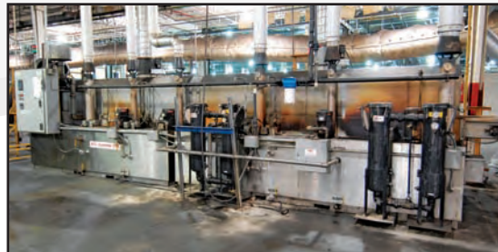
AEC SYSTEMS 6 stage wash line
