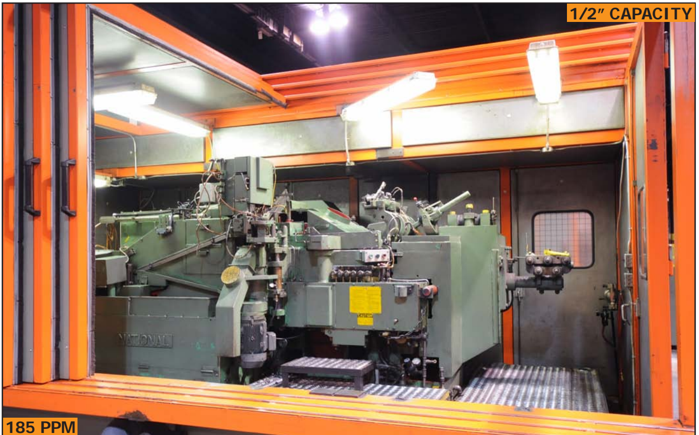
185 PPM NATIONAL 8L4 high speed 4 die bolt maker
