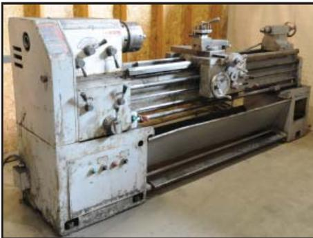
**TAICHUNG** 18/26" X 60" gap bed engine lathe
