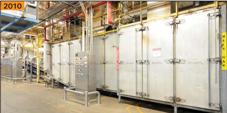
PROCTOR & SCHWARTZ cooked rice S/S dryer oven
