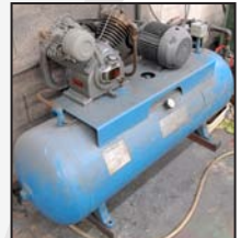
Tank mounted piston type air compressor
