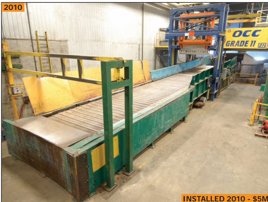
BLACK CLAWSON-NEILSEN & HEIBERT OCC continuous type stock preparation line
