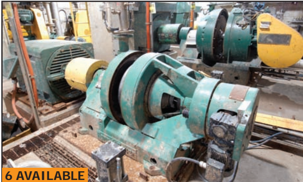
SPROUT WALDRON EM-TYPE II & III refiners 26" & 34"
