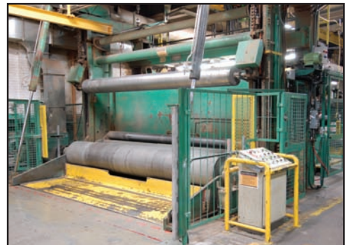
BELOIT M 24-R-60 slitter re-winder
