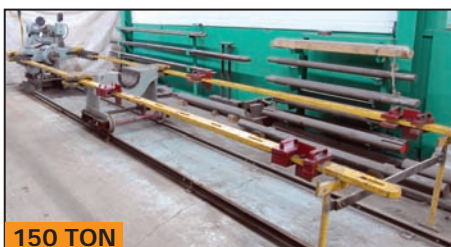
150 TON JAS MORRISON horizontal hydraulic wheel press
