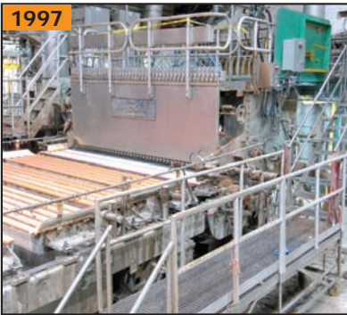
GL&V DR1-16 pressurized type HEADBOX
