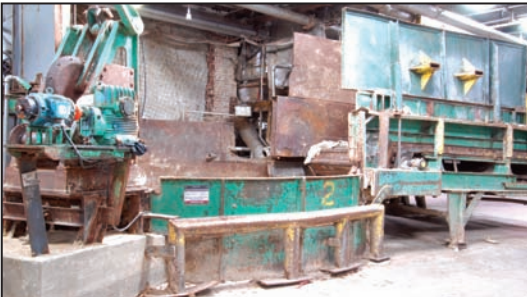
BLACK CLAWSON 20' pulper stock preparation line with SCAVENGER #2
