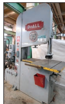
DOALL ZW-3620 vertical band saw
