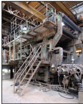
BELOIT Tri-Nip press section
