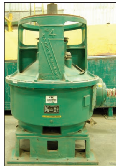
View of spare HYDRAPULPER #4 drive
