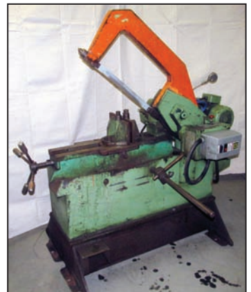
Metal cutting horizontal hack-saw
