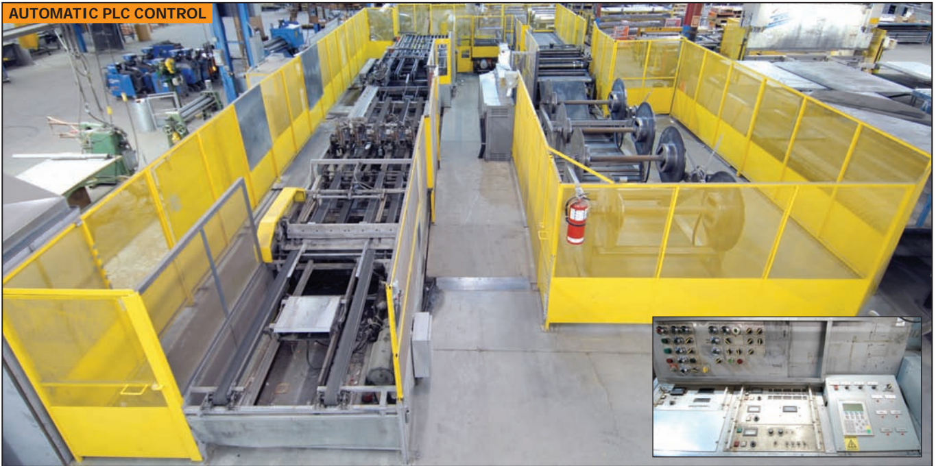
LOCKFORMER-IOWA PRECISION TDC automatic duct panel production line
