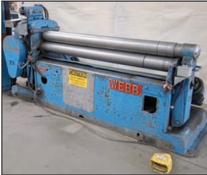
WEBB 505 initial pinch and slip power bending rolls
