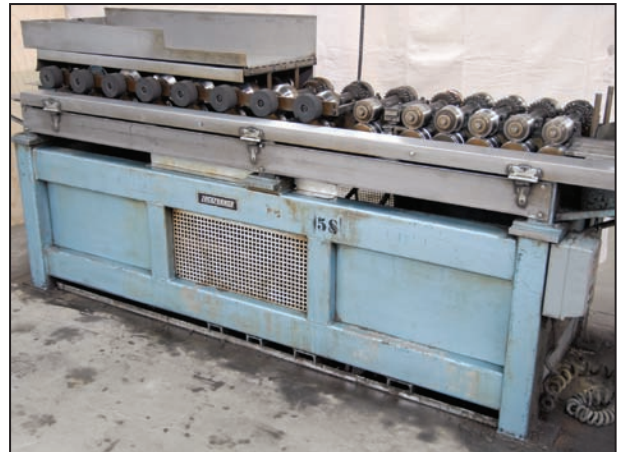
LOCKFORMER TDC transverse duct connector roll former
