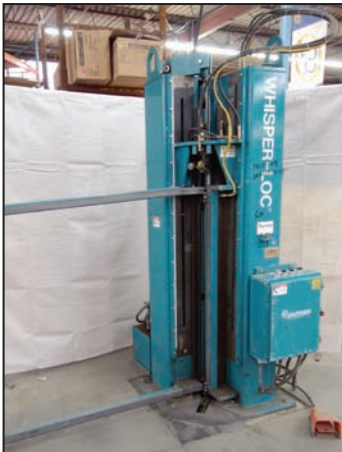
IOWA PRECISION WHISPER-LOC FAH1872-VP duct seam closing machine
