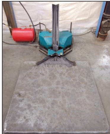
LOCKFORMER CORNER CADET corner and angle inserter
